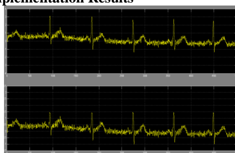
Figure 5: I/P & O/P Waveforms of Chebyshev II filter
